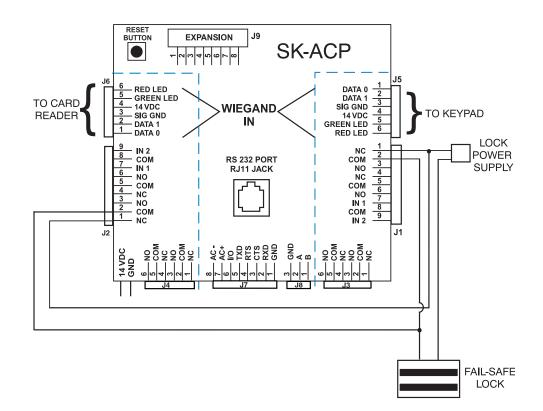
NOTES: Each valid access will appear as two valid access messages in SK-NET. Set the latch timers long enough to allow the user to present his card after entering his PIN and still have time to get the door open.
