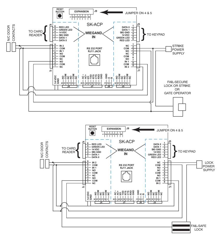
NOTES: Where dual-credential is required during just certain hours or days of the week, you may use the auxiliary output, defined as a "Time Zone" activated, to shunt either the keypad or the card reader during single-credential time periods.
