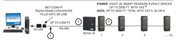
\* NOVA.16 HAS TWO SEPARATELY FUSED 14VDC POWER OUTPUTS - EACH HANDLES MULTIPLE READERS
