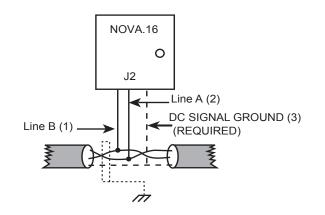
Earth Grounded Shield is highly recommended in environments subject to high voltage electrical discharge (i.e. lightning). Shield should be connected to earth ground only at one end of the cable. DC Signal ground is required. DC Ground wire is NOT to be connected to earth ground.
