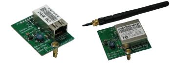
Secura Key's Network Modules allow the SK-ACP to easily connect to your Local Area Network, so that you can use your existing network infrastructure to monitor and control your access control system. You have your choice of SK-LAN-MOD for 10/100 Base-T Ethernet connections or the SK-WLS MOD for 802.11b/g wireless.
