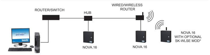
(3) ETHERNET CABLE: (Required cables CAT 5e or CAT 6).
