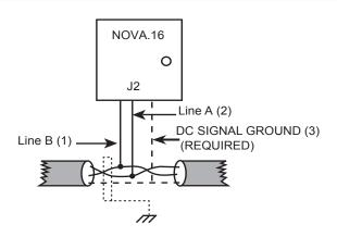
Earth Grounded Shield is highly recommended in environments subject to high voltage electrical discharge (i.e. lightning). Shield should be connected to earth ground only at one end of the cable. DC Signal ground is required. DC Ground wire is NOT to be connected to earth ground.
